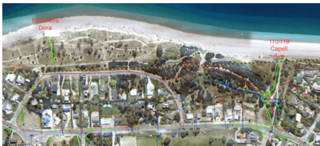
Figure 1 Stormwater drains (green) from Flora Dora Tce to the access to Scott's beach
