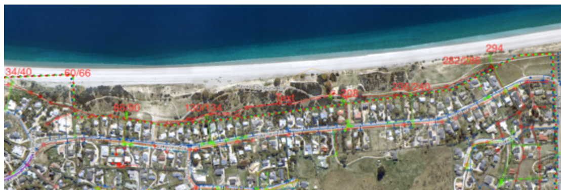
Figure 2 Stormwater drains (green) from Skinner Terrace to Muir Rd
